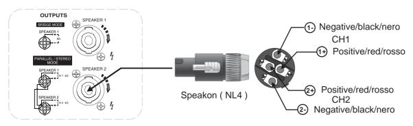
NOTES: The speaker connector can work from 4-16 $\Omega$  in srereo or parallel model. It can work good from  $8\Omega$  to  $16\Omega$  in bridge mode.
