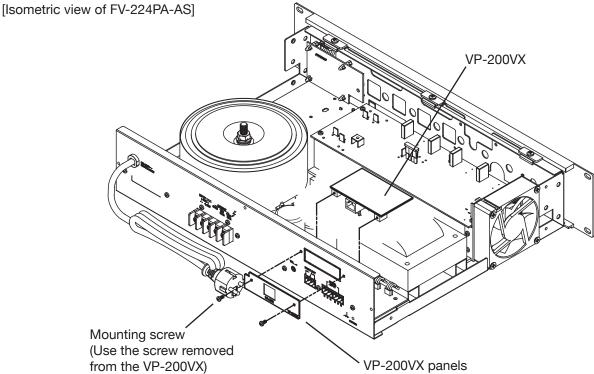
Step 5. Plug the VP-200VX's connector into the connector on the circuit board inside the amplifier.
