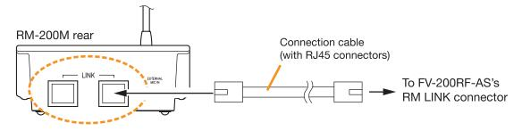
Without AC adapter pluged into RM-200M power will be supplied from system Power Supply trough FV-200RF-AS DC Supply terminal.
