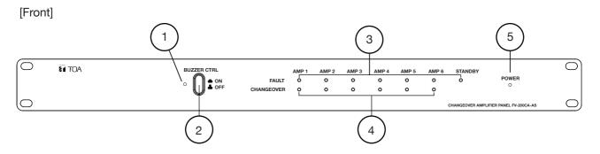
1. Buzzer CTRL Indicator Will light red when Buzzer CTRL switch pull off or buzzer is being muted.
