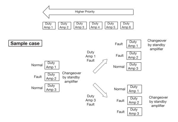
FV-200CA-AS have 7 LED fault indicator for connected amplifier including standby amplifier fault and have 6 LED changeover indicator. Only one LED changeover indicator can light at once, but LED fault indicator will light as many as fault occur at duty or standby amplifier.
