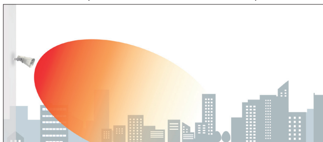
Sound Dispersion of the Conventional Horn Speaker
